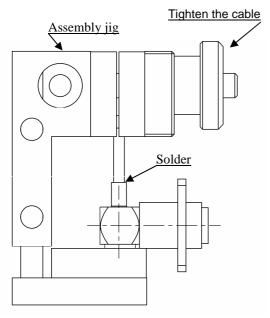
After cooling, remove the assembly from the jig. Solder the inner conductor. Place the cap into the body. Press on the cap flush or slightly below the surface of the body assembly.
